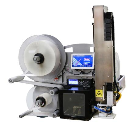
make adjustments as needed during operation. Two compressed air circuits allow the label to stay on the tamp pad and the thruster to stay in position when an emergency stop occurs on the production line. This eliminates the need to reset the applicator when the emergency is cleared and the line restarts.
